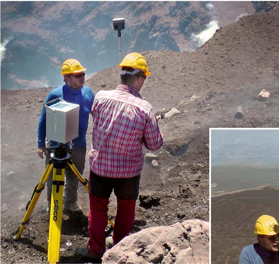
Researchers use Trimble GNSS to locate aerial photo targets and gravimetry points.
